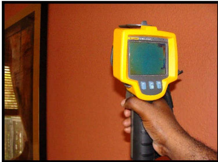
This is a stock photo of a IR or Infrared camera, such a device was used to scan for moisture at your property. Infrared cameras measure levels of infrared light being emitted off surfaces, these levels are translated to temperature readings by the camera that in turn will typically correspond directly to the amount of moisture evaporating off a surface.
