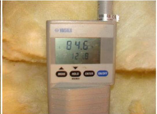
Temperature humidity and grains of moisture were high in the attic.
