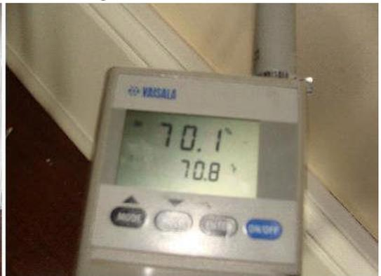
Temperature humidity and grains of moisture were high in the partition walls and in the perimeter walls that abut the exterior. Above is a perimeter wall with humidity problems inside. Circle indicates where measurement was taken of inner wall air.
